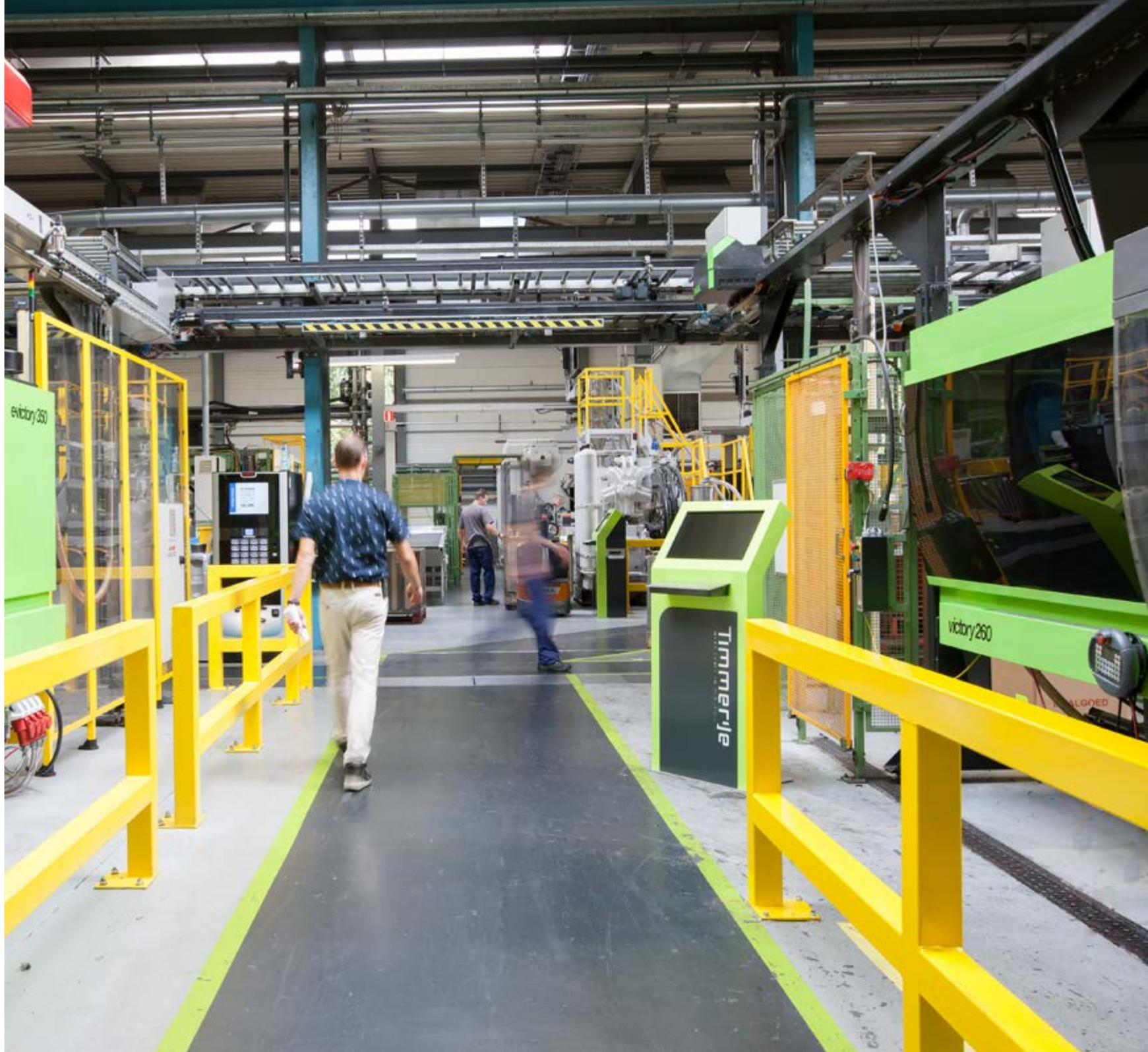
The wide range of injection moulding machines enables client-specific plastic components to be manufactured.
